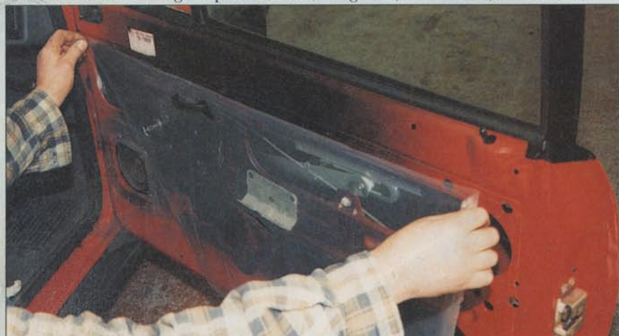
12. Finally, a sheet of plastic covers the inside of the door to protect the casing from any stray damp that might be floating around.
