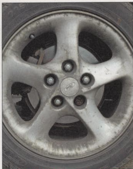
1 Pretty Probe wheels were in a horrible state, most likely as a result of silver paint being applied directly on to the alloy surface without any primer. As well as flaking lacquer, there was also extensive kerbing damage to the outer rim.
