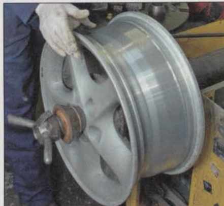
6 In a different part of the workshop the wheels are spun up by hand and checked for trueness, cracks and distortion. The vast majority of buckles can be corrected by the use of localised heat and a mallet.
