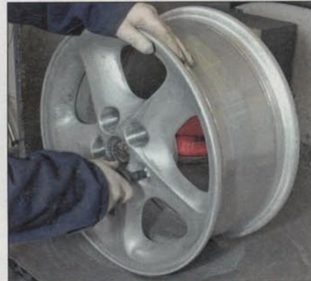
7 If given the okay the wheels are cleaned up with various abrasive tools to remove any stubborn deposits. It also serves to 'key' the alloy surface ready for the application of the powder coat primer.
