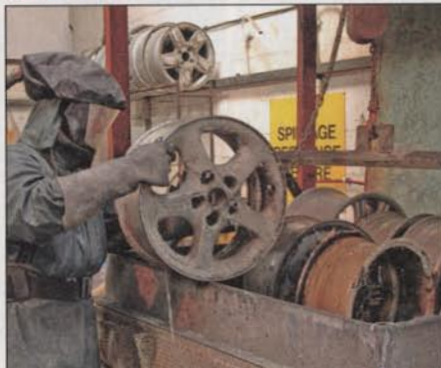
4 Once the tyres had been marked up and removed the wheels were put into a chemical stripper for three hours to remove all the old paint and lacquer. It's eco-friendly Benzol Alcohol, not hydrochloric acid. The bigger overnight stripper takes a staggering 60 wheels!
