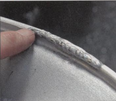
8 One of the Probe wheels had a particularly nasty parking ding in the rim so the area around it was ground away to remove any foreign objects before a build up of TIG weld was applied.
