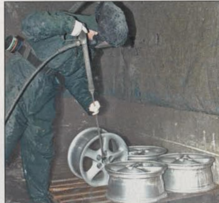
5 Once out of the stripper the wheels are thoroughly jetwashed to remove all the mucky deposits. Full protective gear is essential while doing this as the fumes are suffocatingly bad.
