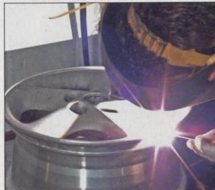
8 One of the Probe wheels had a particularly nasty parking ding in the rim so the area around it was ground away to remove any foreign objects before a build up of TIG weld was applied.
